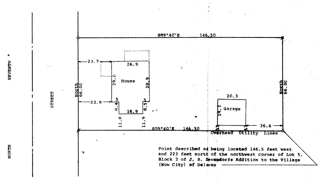
Scale - 1" = 20' # 1" Iron Pipe Found 0 = 3/4" Iron Pipe Found Bearings referenced to the assumed bearing of North along the east line of North 7th Street Survey ordered by: Myron Mathison 197 North 7th Street Delavan, WI 53115
